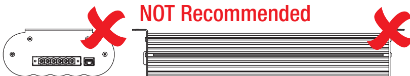
Figure 2.2.1.3 - Do NOT mount the unit upside down
