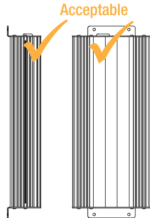
Figure 2.2.1.2 - Vertical mounting is acceptable
